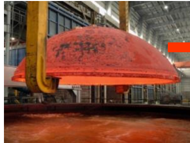
heat treatment of the top head
