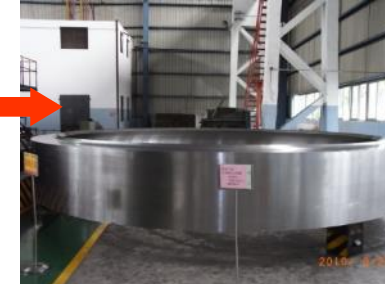
fine machined top flange
