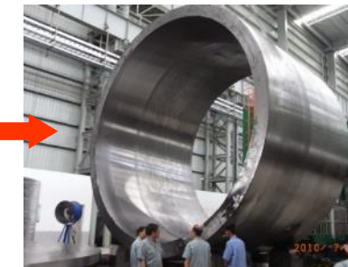
preliminary machined large forgings
