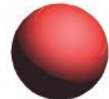
Uranium Dioxide Kernel, Dia. 0.5mm
