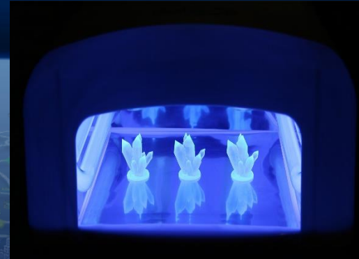
Ultraviolet Curing (Replaces Heat)
