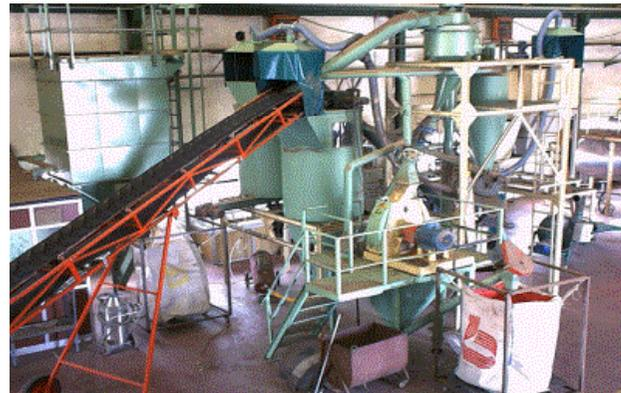
Pilot plant for granule-metric reduction of biomass, 200-700 kg/h
