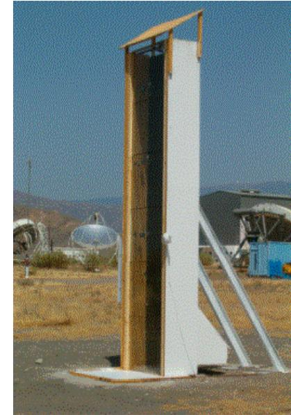
Solar chimney prototype for testing at PSA
