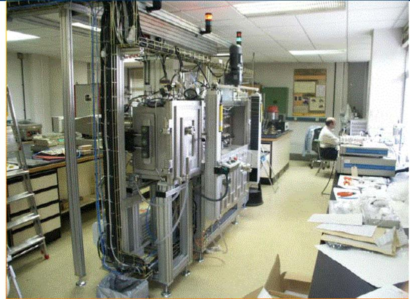
Micro-pilot plant of cathode spraying to processing 30 x 30 cm samples
